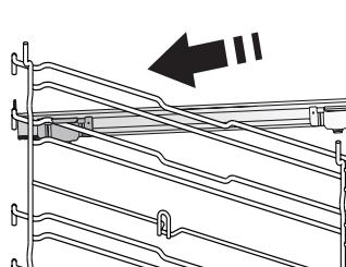
Remove the shelf guides from the oven and remove the protective plastic from the sliding runners.
