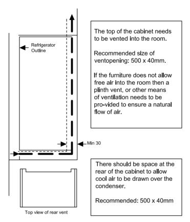
The open channel at the rear is clearly shown. For the correct operation of the appliance it is important that the top of the housing unit is not blocked off. A channel depth of 40-50mm is normal with most units.
