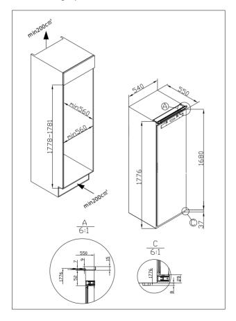
An air intake should be provided somewhere in the cabinet run to allow free air in. in this example,a plinthvent is shown underneath the refrigerator.
