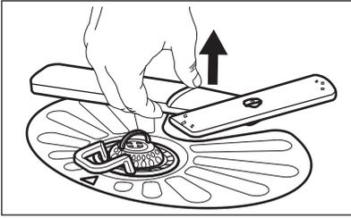
2. Wash the spray arm under running water. Use a thin pointed tool, e.g. a toothpick, to remove particles of soil from the holes. Run water through the holes to wash soil particles away from the inside.
