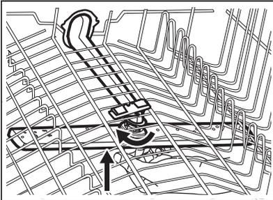
3. Wash the spray arm under running water. Use a thin pointed tool, e.g. a toothpick, to remove particles of soil from the holes. Run the water through the holes to wash soil particles away from the inside.
