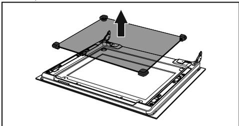
N.B.: in some models, the intermediate glass unit consists of two glasses.
