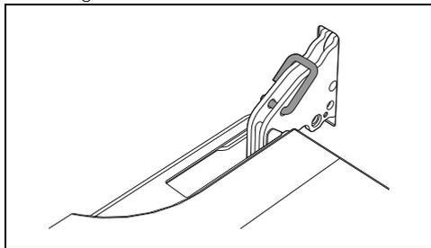
2. Grasp the door on both sides with both hands, lift it forming an angle of around 30° and remove it.
