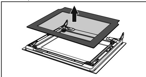
5. Remove the intermediate glass unit by lifting it upwards.
