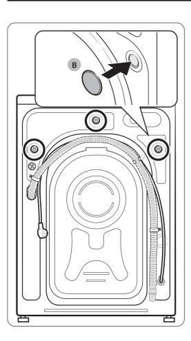
**3.** Insert the **bolt caps (B)** to the holes (marked with circle in the figure).
