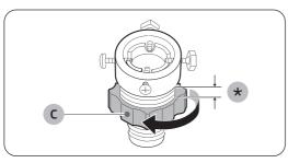
**3.** Hold the adaptor and turn **part (C)** in the arrow direction to loosen it by 5 mm (\*).
